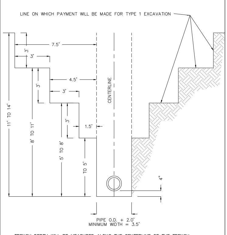
TRENCH DEPTH WILL BE MEASURED ALONG THE CENTERLINE OF THE TRENCH AT DEPTHS EQUAL TO THE VERTICAL DISTANCE FROM THE FINISHED GROUND SURFACE, OR TOP OF PAVEMENT, TO THE FLOW (INVERT) LINE OF THE PIPE PLUS THE THICKNESS OF THE PIPE BARREL AND BEDDING MATERIAL.
