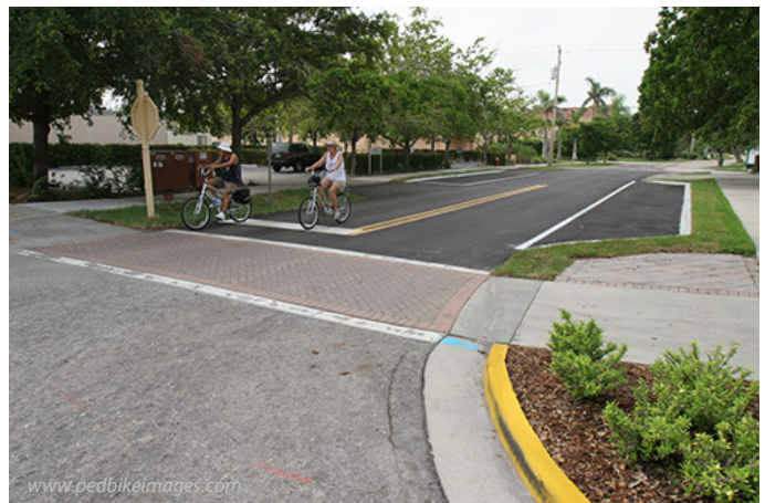
Bulb outs shorten the distance for pedestrians to cross the street.
