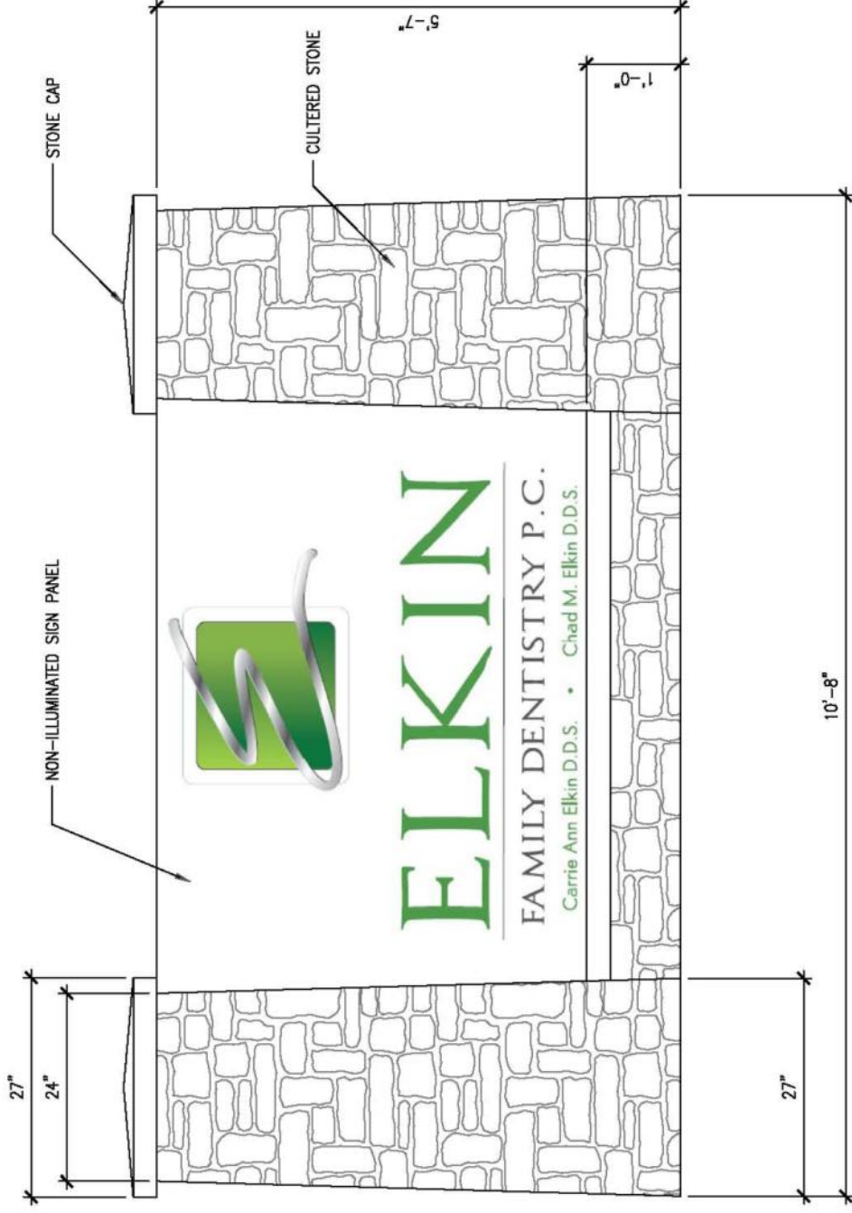
3 SIGN ELEVATION Scale: 3/4"=1'-0"
