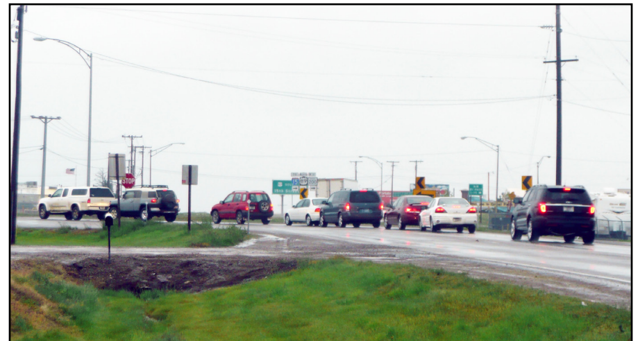
The intersection of Bootlegger Trail and US-87 operates at a failing LOS during the PM peak hour.
