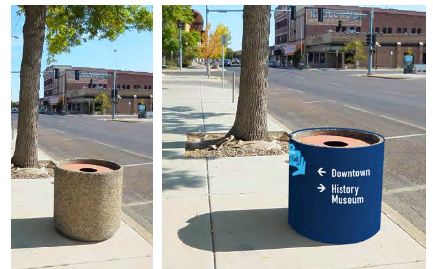
Waste receptacle steel slip collar concept with wayfinding brand implemented
