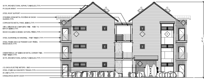
2 SOUTH ELEVATION - DRB DRB1.5 1/8" = 1'-0"
