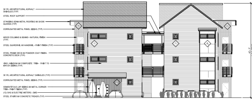
3 EAST ELEVATION - DRB DRB1.3 1/8" = 1'-0"
