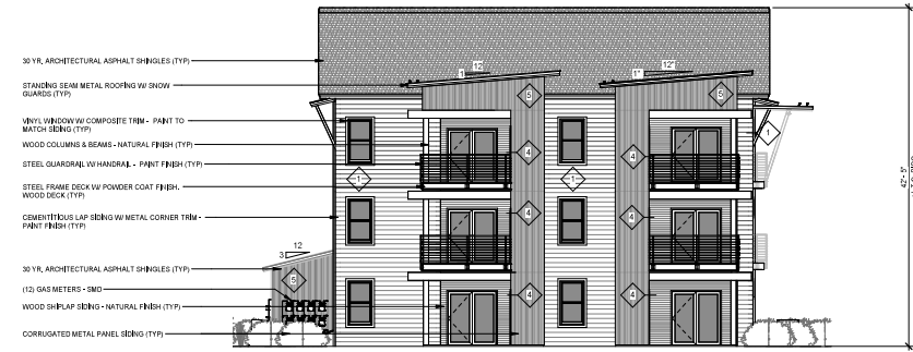
3 EAST ELEVATION - DRB DRB1.5 1/8" = 1'-0"
