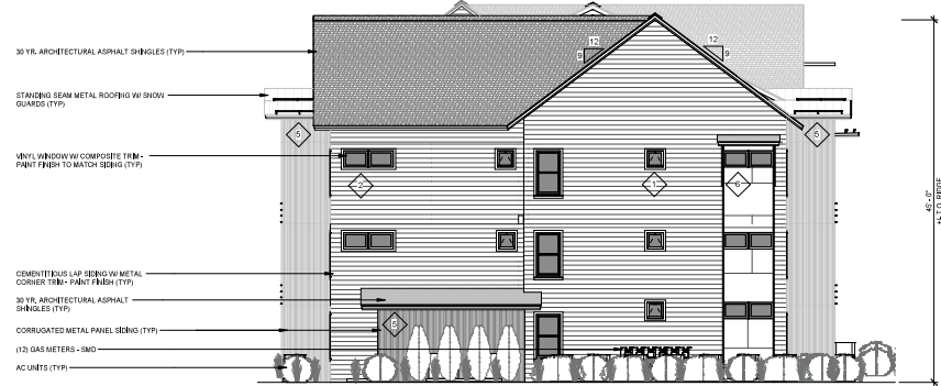
3 EAST ELEVATION - DRB DRB1.6 1/8" = 1'-0"
