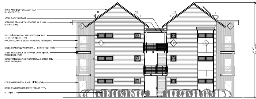
1 NORTH ELEVATION - DRB DRB1.5 1/8" = 1'-0"
