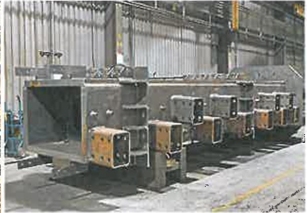
Complex and heavy built-up steel components Column of the EnCana building, in Calgary
