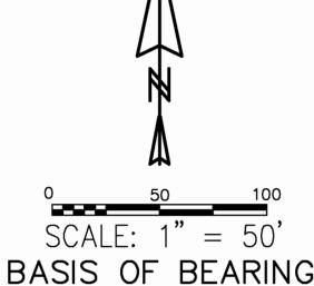
BASIS OF BEARING IS TRUE NORTH BASED ON GEODETIC INVERSES USING SURVEY GRADE G.P.S. SYSTEM.
