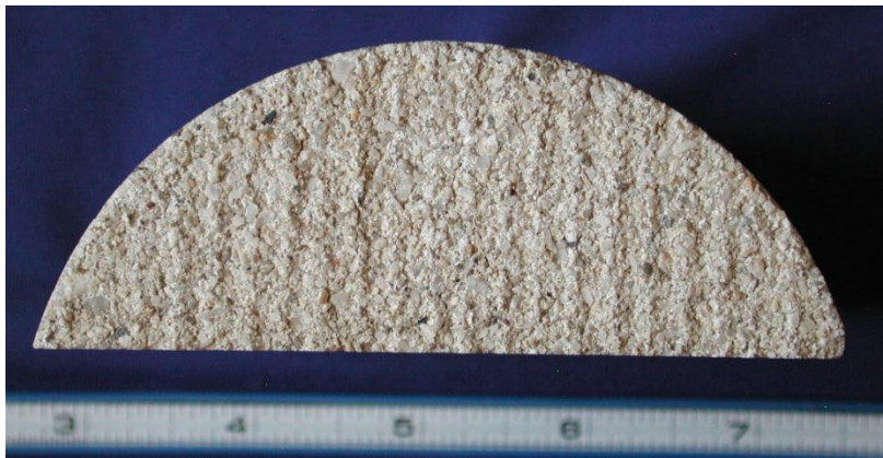
Figure 6. View of the finely ridged, exposed surface of the face mix.
